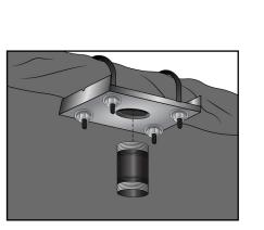
**Step 7** Attach the extension column to the center hole.
