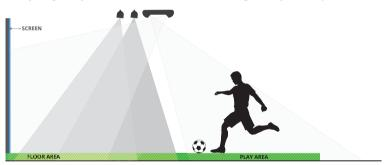
See the previous page for instructions on installing a single IR Booster Light. When installing a second light, it should be clamped/attached immediately in front of and in line with the first light.
