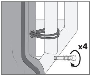
Alternate tightening each end of the cable. Use a pliers to hold the cable and prevent it from spinning, while using 3/16" Hex key to tighten the receiver.
