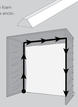
When you get to the end, trim off excess foam using a cutting tool. Make adjustments to smooth out the flaps and tuck in the corners for a neat fit.
