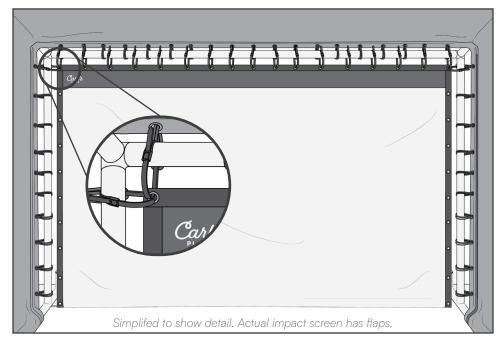
Next, you'll attach the bottom of the impact screen using the cable. The cable is pre-threaded through the bottom sleeve of the impact screen.
