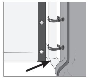
On one side, insert the cable through the fitting.
