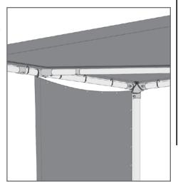
Next hang the wall panel marked with 2 blue tabs. Orient with the 2 blue tabs to the rear left top. Again, slide the bottom sleeved edge of the panel onto the bottom pipe.
