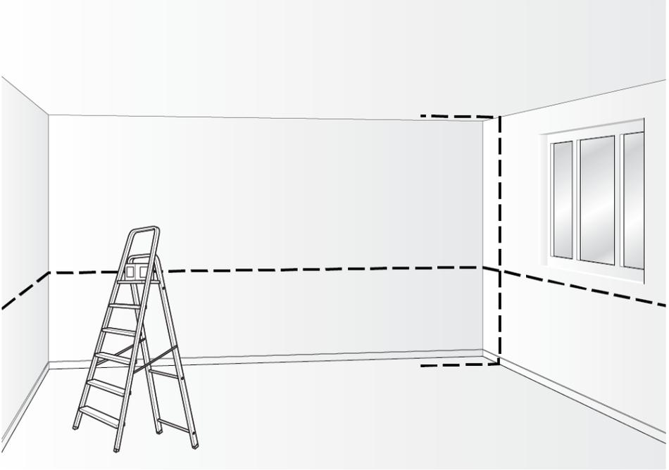
Use a laser level to align all components for your golf simulator. Ensure they are set on an even plane, perpendicular to the side walls. Plan to place the screen at least 1 foot from the back wall to allow for fast-flying golf balls.
