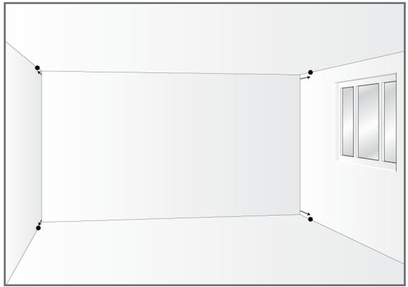
Set one corner cable anchor in place on the floor with the tapered end pointing up.
