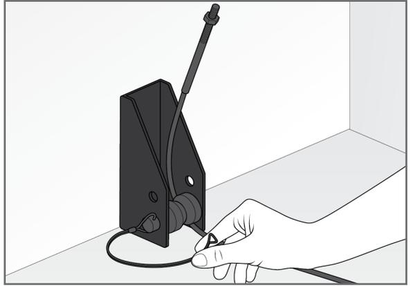
Connect the top and bottom cable ends together on each side via the turnbuckles and tighten just until cable system is taut. **Do not overtighten.**
