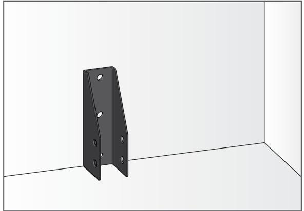
Make sure the corner cable anchor is level. Then mark the bottom angled hole and drill a pilot hole at a downward angle for the ¼" lag screw. Use one screw to secure it in place through the bottom angled hole into the bottom plate of the wall.
