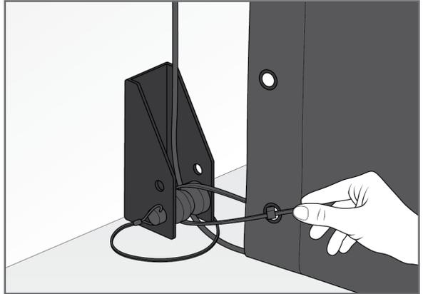
With the corner grommets secured and the cable tensioned just until taut, use zip ties through all other grommets and around the cable.
